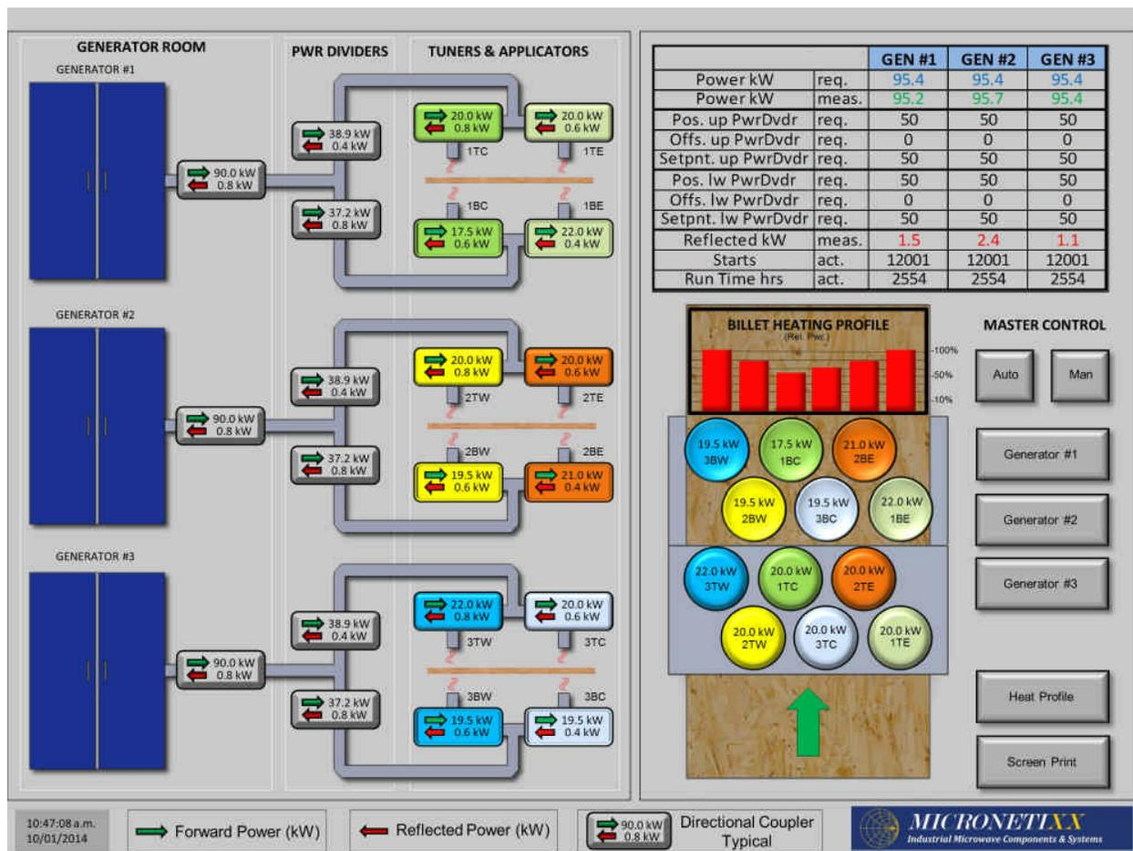
An Example of an HMI Screen for the *Visuex<sup>tm</sup>* Micronetixx LVL or MDF System Up-Grade
