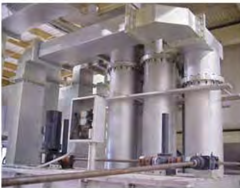
High Power Microwave Engineered Lumber Heating System
