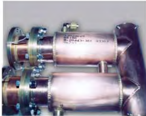
Water-Cooled Coaxial Low-Pass Filters
